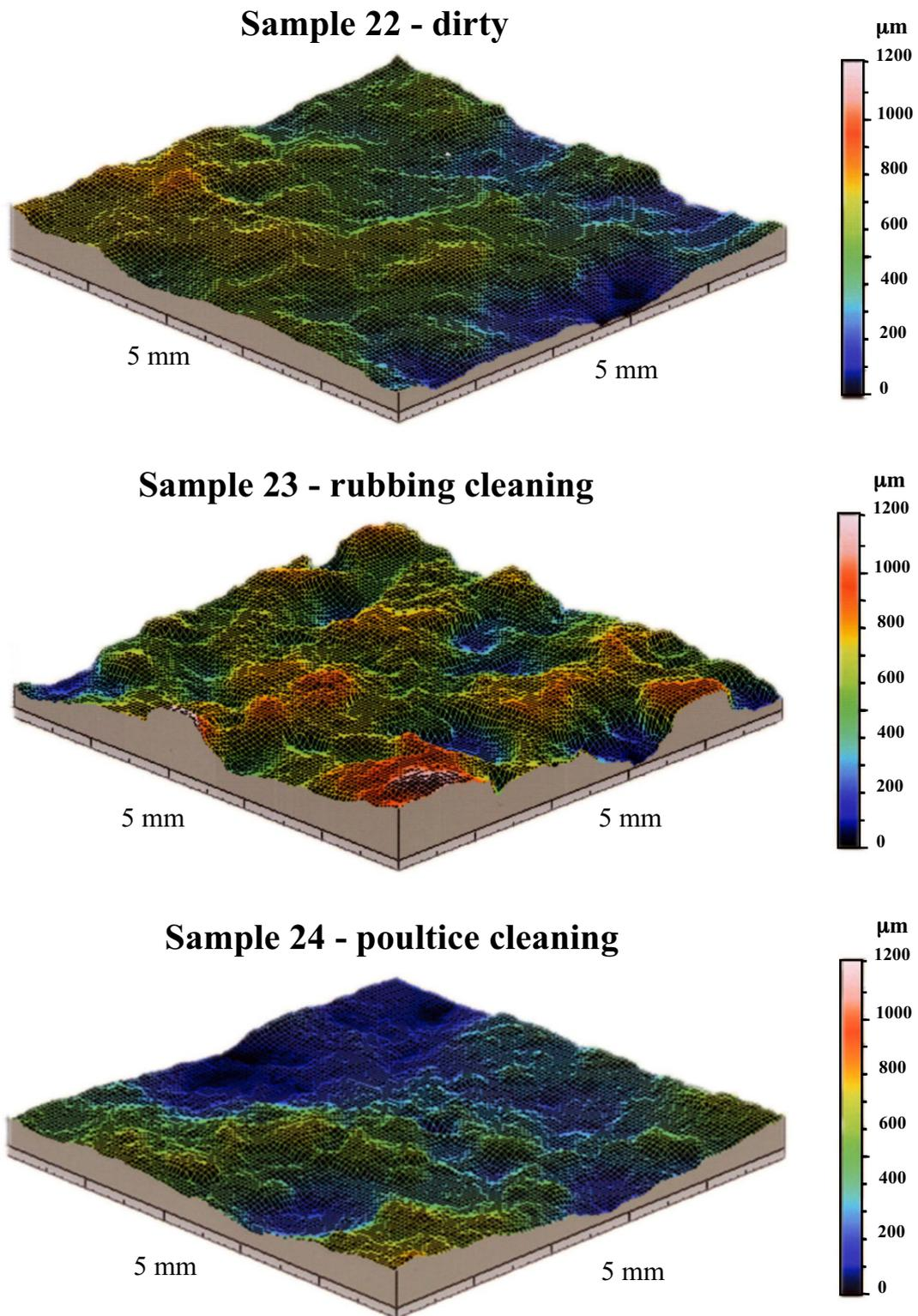
Figure 5. Surface 3d reconstructions of the studied samples.
