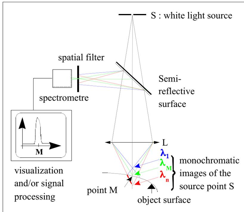
Figure 2. Principle of the extended field confocal microscopy (after Cohen-Sabban, 1999)
