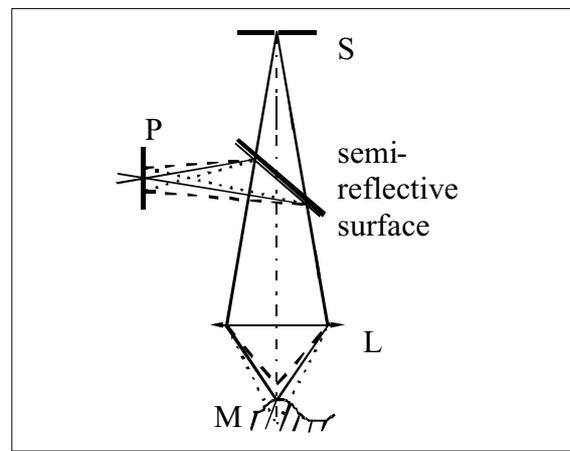
Figure 1. Principle of the confocal imagery (after COHEN-SABBAN, 1999)
